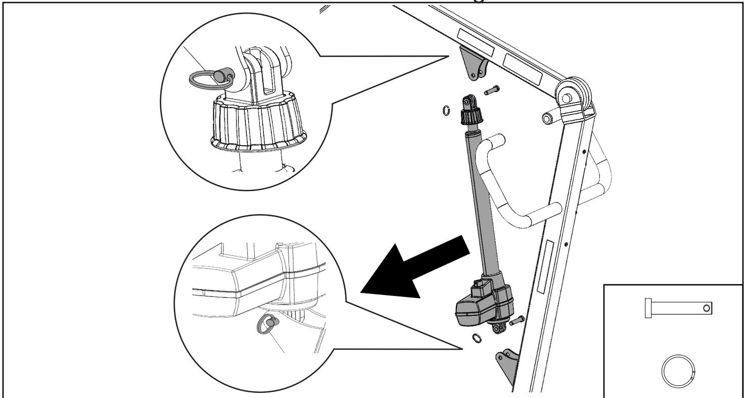
Step 8: Secure the spreader bar to the boom using a pin and retaining ring as follows.
