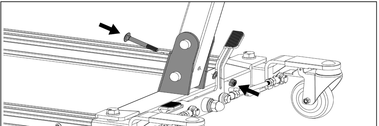
Step 4: Insert the round plastic cover and the large plastic washer to the boom as follows.
