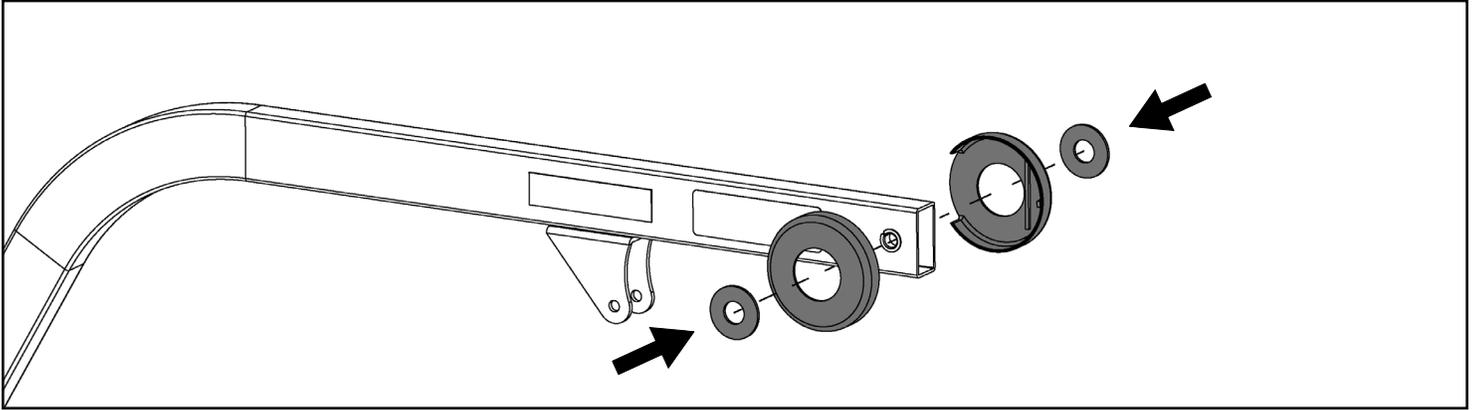
Step 5: Install the boom to the mast bracket, and make sure the plastic cover and plastic washers are still attached to the boom.
