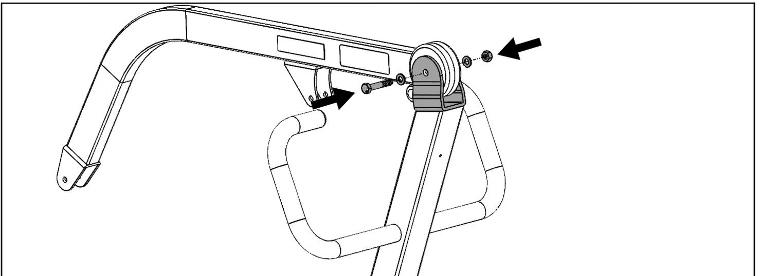
Step 7: First, secure the lower end of the actuator to the bracket on the mast using a pin and retaining ring. Then, secure the upper end of the actuator to the bracket on the boom using a pin and retaining ring as follows. It is critical to have the motor part of the actuator to face the same direction as the big arrow as follows.
