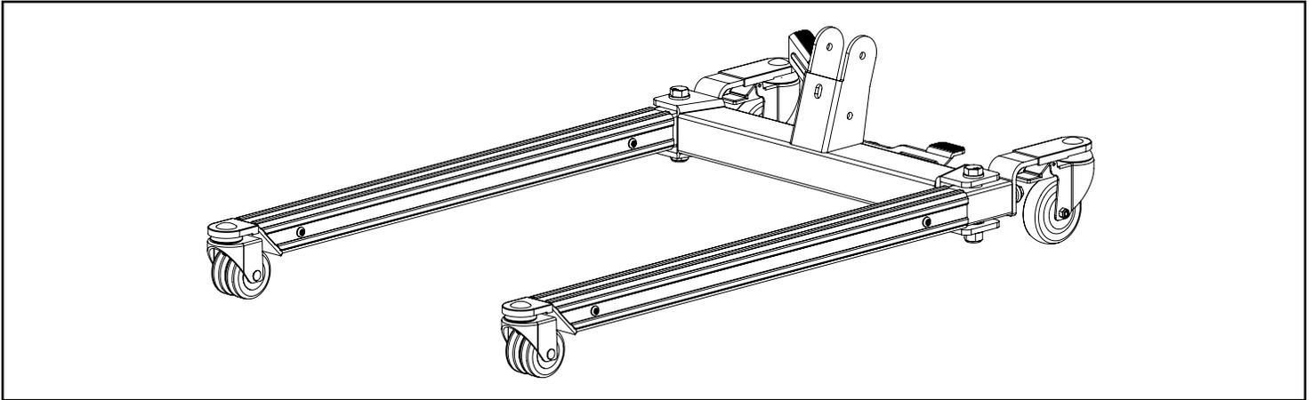
Step 2: Insert the mast and align the side holes on the mast with the holes on the bracket. Secure the mast to the bracket using the side bolts and cap lock nuts.
