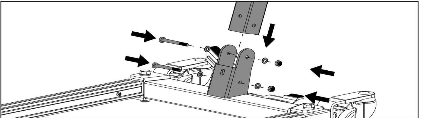
Step 3: Insert the carriage bolt to the front hole of the bracket, and secure the mast using bolts and cap lock nuts as follows.
